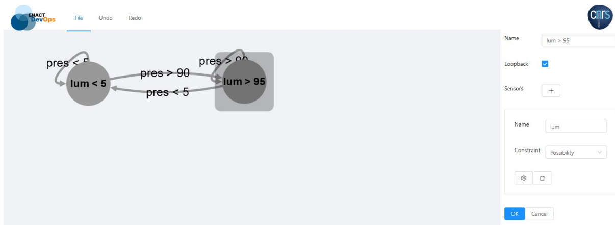
Figure 12: Deterministic model describing the expected evolution of physical model (relation between luminosity and presence in the room)
